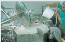
Mixing Mixing surimi and ingredients with silent cutter
